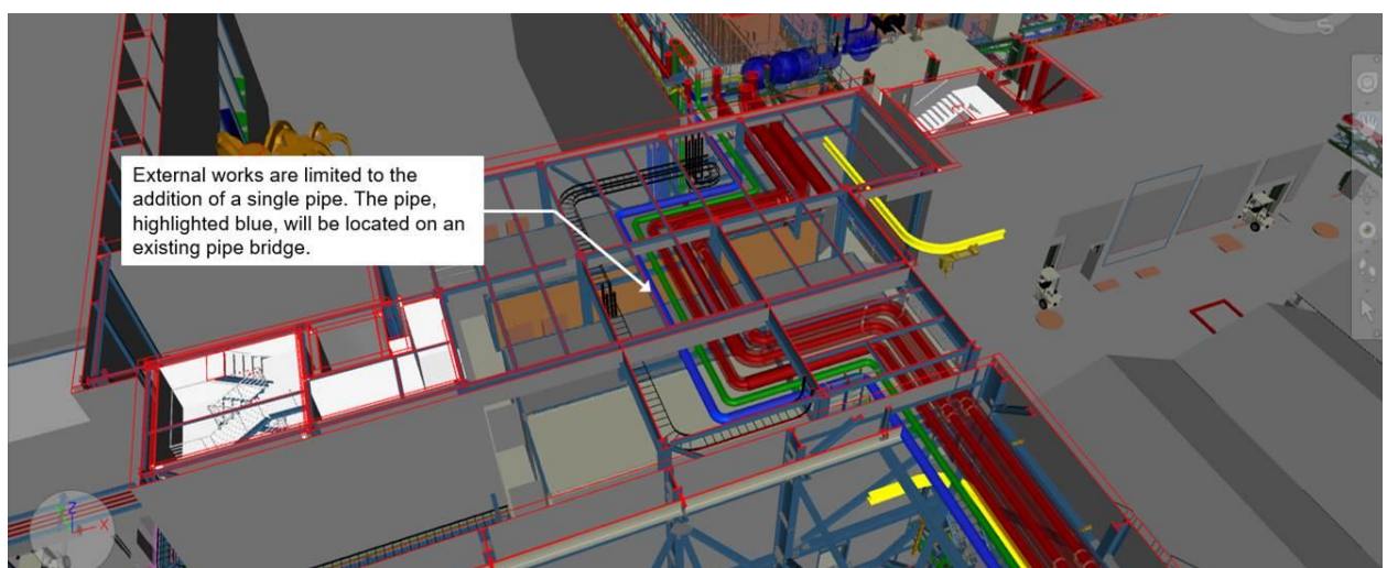
Plate 2.2 – 3D Model Close-up Aerial View of Consented Development with external pipework and pipe supports (Note – Proposed Project external pipework is coloured blue)
